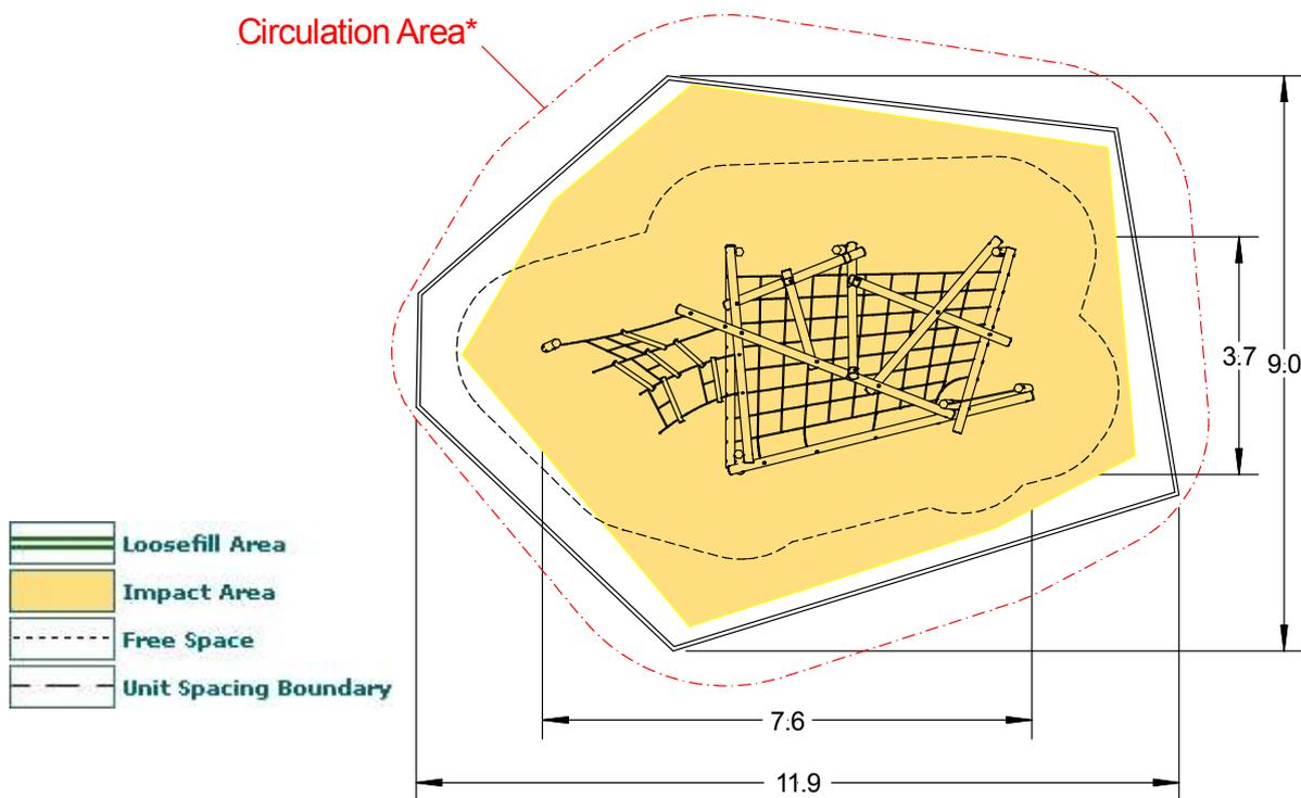
\* Recommended Circulation Area (1.2m outside impact area) – this area should be clear of solid raised objects (ie.fences, walls, trees and other items of equipment). Loose fill retaining edgings are acceptable in this area.
